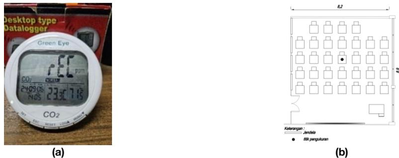
**Gambar 1.** (a) CO<sub>2</sub> Temperature RH Indoor Air Quality Monitor Data Logger; (b) Penempatan Alat Pengukuran.
