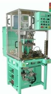
Gambar 2. *Leak Tester Machine*.
