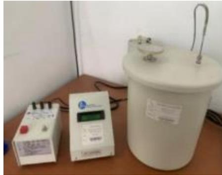
**Gambar 3.** Kalorimeter bom.
