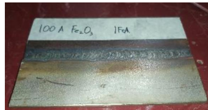
Gambar 3. Visual hasil lasan 100 A activated flux \text{Fe}_2\text{O}_3
